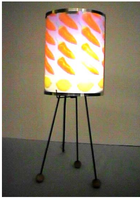
Figure 3. The Lampshade intentional presence device. The local user has chosen to be represented by lemons, seen in the lower part of the lampshade, and the remote user has chosen chili peppers, seen in the upper part. Both users have intentionally indicated their presence.
